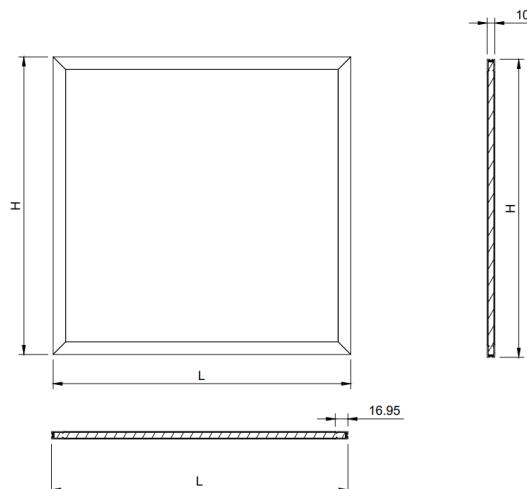
G4 air filter with frame, made of aluminum, used for air filtration and mounting on the ceiling diffuser connection.
