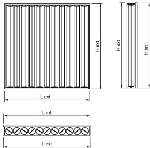
The damper is equipped with opposable blades and is mounted on the ceiling diffuser connection for adjusting the air flow.
