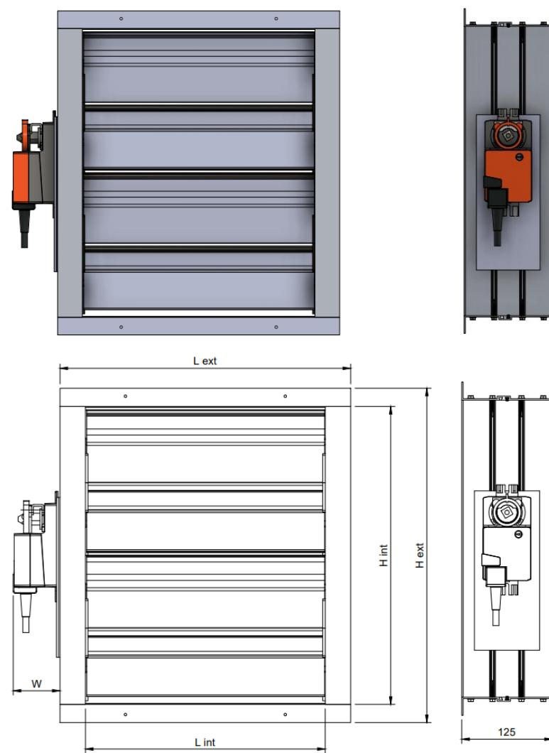
The servomotor mounted on the VCD-S is ordered separately.
