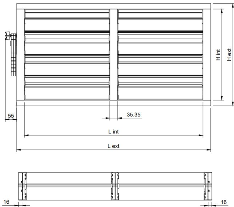
Electrically operated dampers with an area  $\geq 4 \text{ sqm}$  require 2 servomotors according to the drawing.
