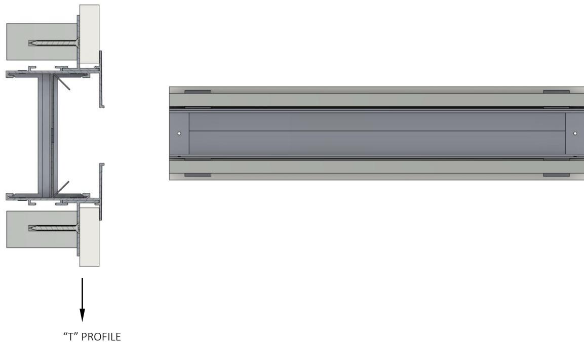
The "T" profile is ordered together with the LENOX diffuser and is installed by the manufacturing department in the diffuser. The positioning of the "T" profile on the diffuser channel is done according to the thickness of the gypsum board (12.5 or 9.5 mm). The gypsum board thickness is specified by the customer when ordering.
