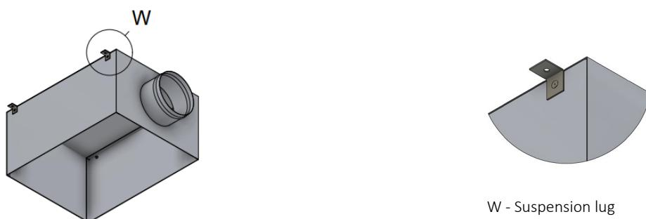
The plenum is available in two options, uninsulated or insulated with 6 mm thick elastomeric rubber.
